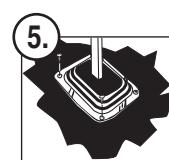
Position retainer plate into place and fasten with sheet metal screws supplied in package.
