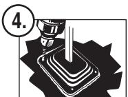
Slide the boot over the stick. Drill 1/8" diameter holes through floor using the boot holes as a guide.
