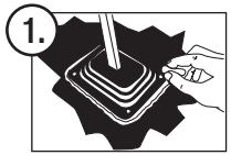
Remove shifter knob. Place boot over stick and slide down to floor. Mark an outline of the boot on the carpet.
