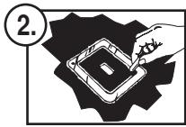
Remove boot and place retainer plate inside the marked outline. Mark the inside opening of the plate on the carpet.
